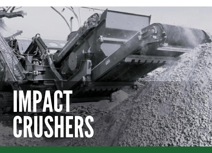
McCloskey brings high quality and high production capacity to mobile impactor applications. The direct drive crusher boosts power and lowers fuel costs, and along with an optimized material flow path and open chassis for ease of maintenance, boosts production and efficiency as well.
