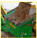
Hopper 14ft (4267mm) grid opening allows the use of larger loading shovels.
