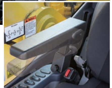
Armrest with simple height adjustment
