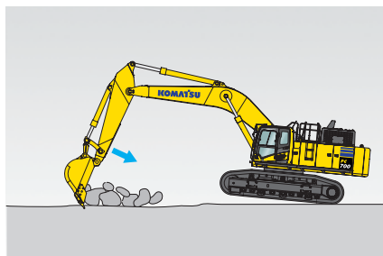
Power mode Boom pushing force is increased, ditch digging and box digging operation on hard ground are improved.
