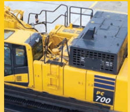
Hand rails and anti-slip plates
