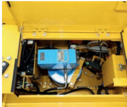
Motorised grease gun equipped with hose reel
